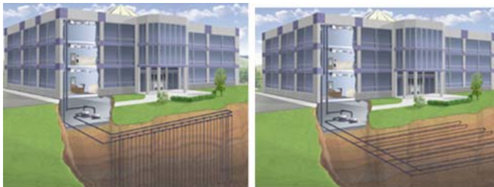
Figure 2.2-a Vertical (left) & Horizontal (right) Closed Loop
